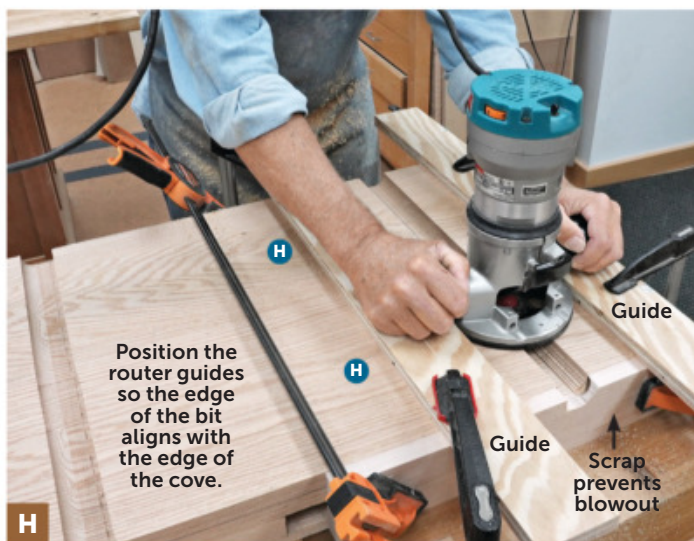
Install a 1\frac{1}{2} " core box bit in your router and measure from the edge of the bit to the edge of the base. Clamp the bases (H) together with scrap on each edge, then clamp guides in place and rout the cove.
