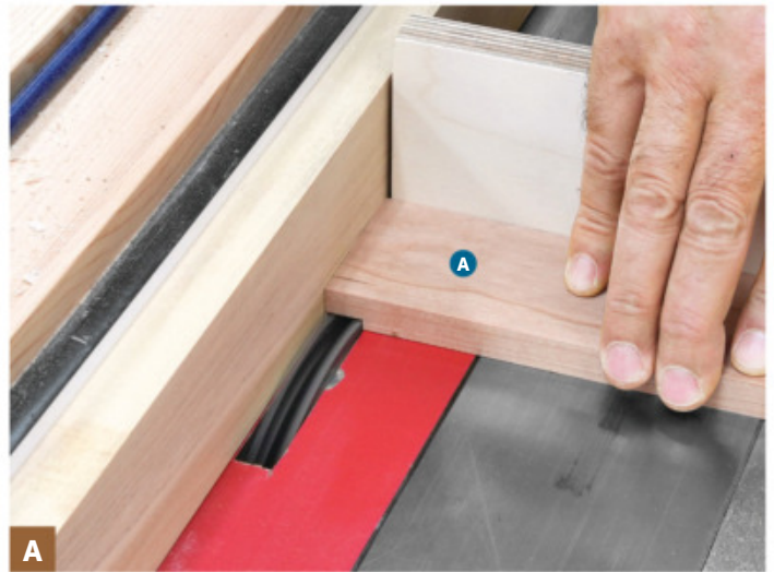
Using a dado blade and auxiliary rip fence, rabbet the ends of the sides (A). An auxiliary fence attached to the miter gauge backs up the cut to prevent tear-out.
