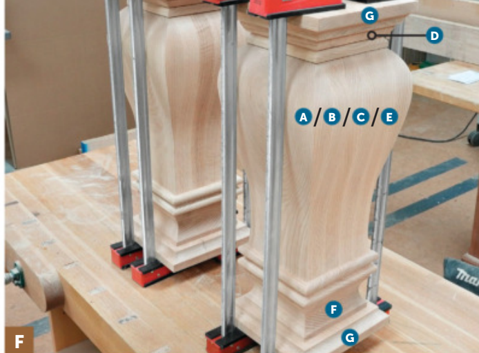
Glue the additional layers—the cove blocks (F), the large chamfer blocks (D), and fillet blocks (G)—to the pedestal assembly. Keep glue about \frac{1}{8} " from the edges of each block to minimize squeeze-out.
