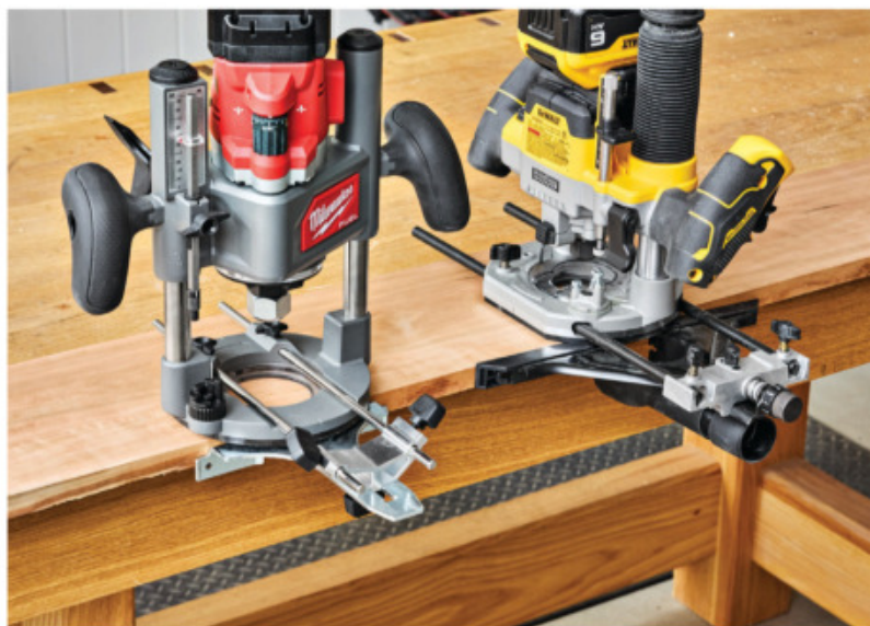
The Milwaukee router places the handles parallel with the edge guide face, which felt awkward in use. The DeWalt, Makita, and Metabo routers orient the handles 90° to the edge guide.
