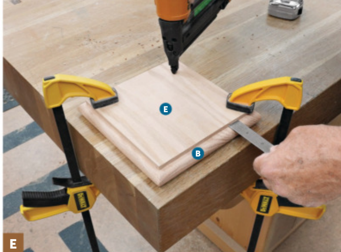
Spread glue on one face of a flat block (E), center it on a bullnose block (B). Use a pin nailer or wire brads to fasten the pieces together. Repeat the steps for the remaining flat and bullnose blocks.
