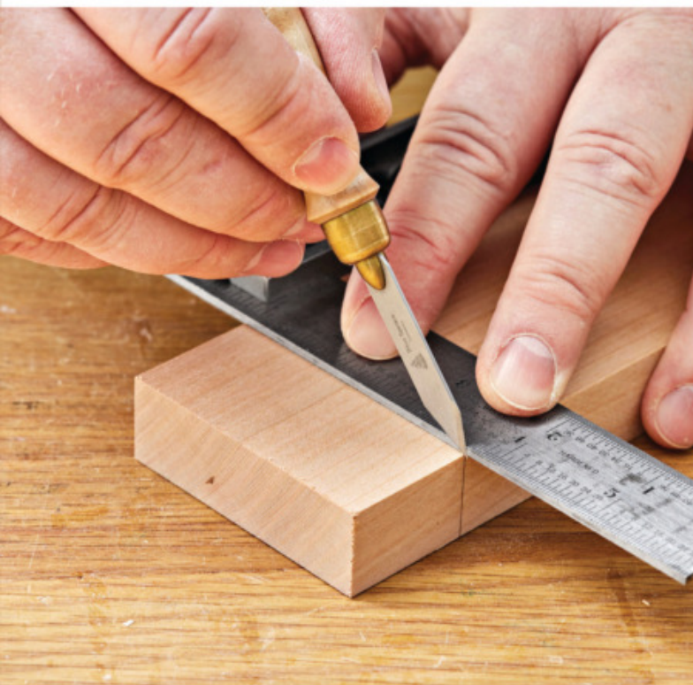
Place the tip of the marking knife into the scribed line you just made and butt the blade of the square against the knife. Scribe a line on one face of the workpiece. Repeat for the other face, then the final edge.
