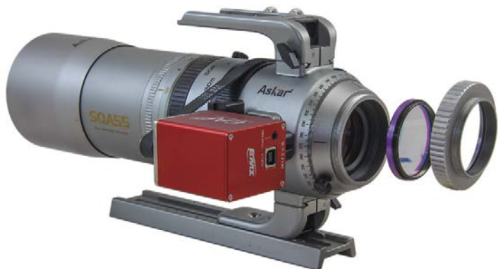
▼ Left: The final adapter ring steps down from the focuser's male M59 threads to present male M48 threads for attaching a camera or T-ring. The adapter ring accepts 48-mm filters. The single rear element of the quintuplet set sits just inside the focuser. Right: From left to right is the silver aperture ring for stopping down the lens, as well as the helical fine-focus ring and the wider coarse-focus ring, both with locking knobs. At far right is the 360° camera rotator with four index lines and markings at 1° increments.
