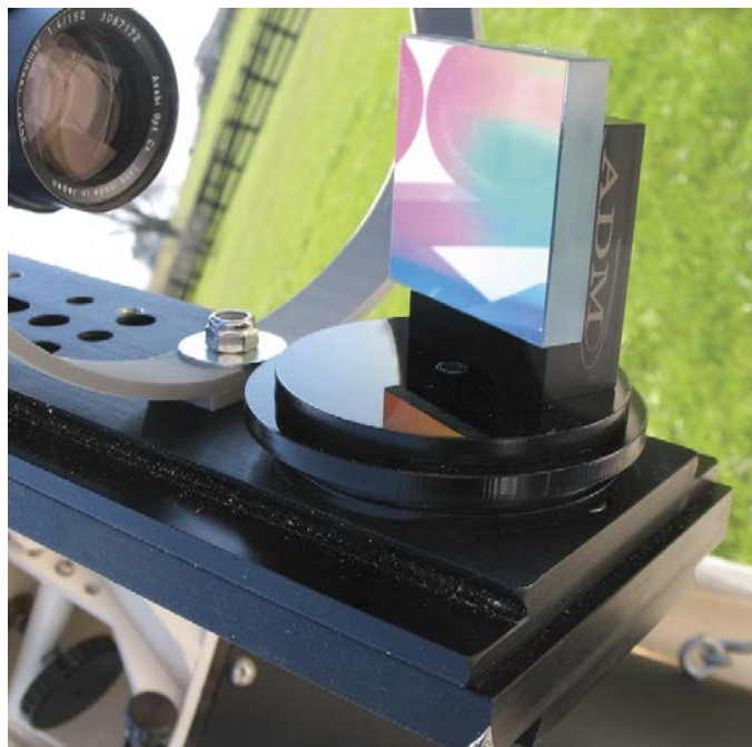
▲ ROTATING GRATING The 2,400-lines-per-millimeter reflective holographic diffraction grating is attached to part of a repurposed ADM V-Series dovetail adapter mounted on a series of acrylic disks used to center the grating in the optical path. The front surface of the grating must be aligned with the rotational axis of its mounting screw.
