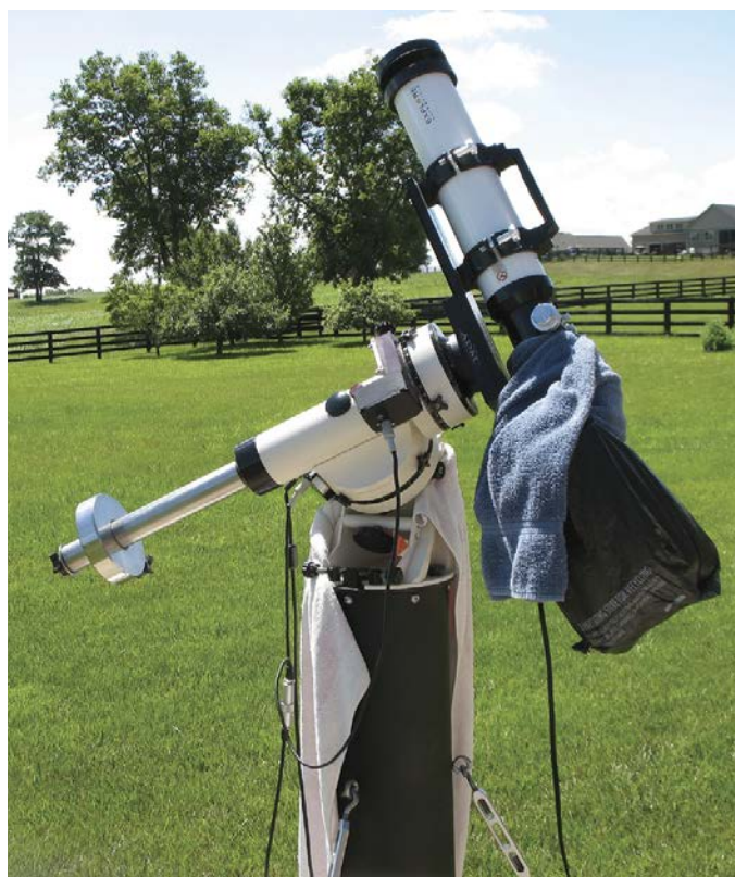
▲ LIGHT-TIGHT The spectroheliograph needs to be sealed from extraneous light while in use. The author uses three nested black plastic bags secured by twist ties, which are then covered with a thick towel.
