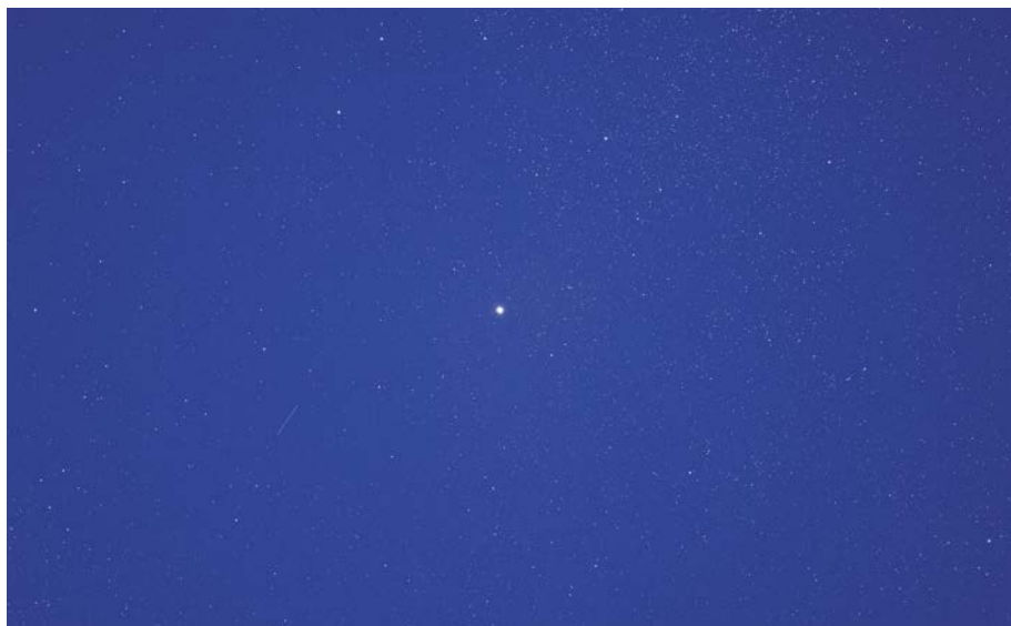
▲ Taken in deep twilight, this 30-second exposure of the sky around Deneb, Alpha ( \alpha ) Cygni, illustrates the SQA's mild, gradual light falloff toward the corners. Contrast has been boosted considerably, as it would be for most deep-sky images.
